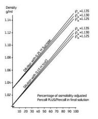
Fig 1. Dilution of stock osmolality adjusted Percoll PLUS/Percoll (340 mOsm/kg H2O) with saline or sucrose solution. p0 is the density of Percoll PLUS/Percoll from the bottle.
